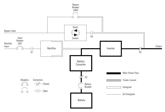
NOTE On an UPS configured as an IOM, the bypass input, static switch, bypass breaker (CB4), and K5 are not present.
